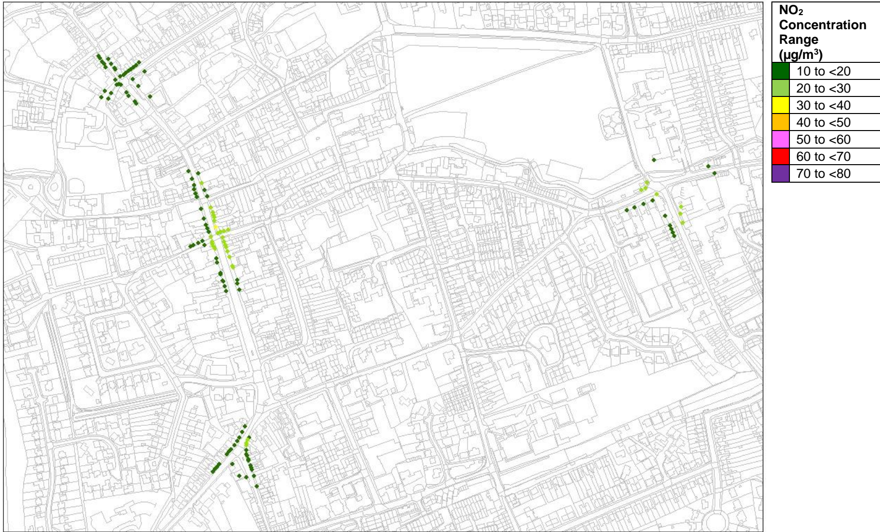
Figure 6-K: 2026 Do Minimum Scenario – Modelled Annual Mean NO 2 Concentrations (based on the LAQM TG09 Methodology)
