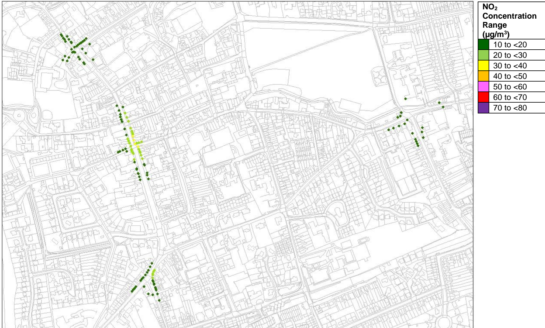
Figure 6-M: 2026 Full Scheme Scenario – Modelled Annual Mean NO 2 Concentrations (based on the LAQM TG09 Methodology)
