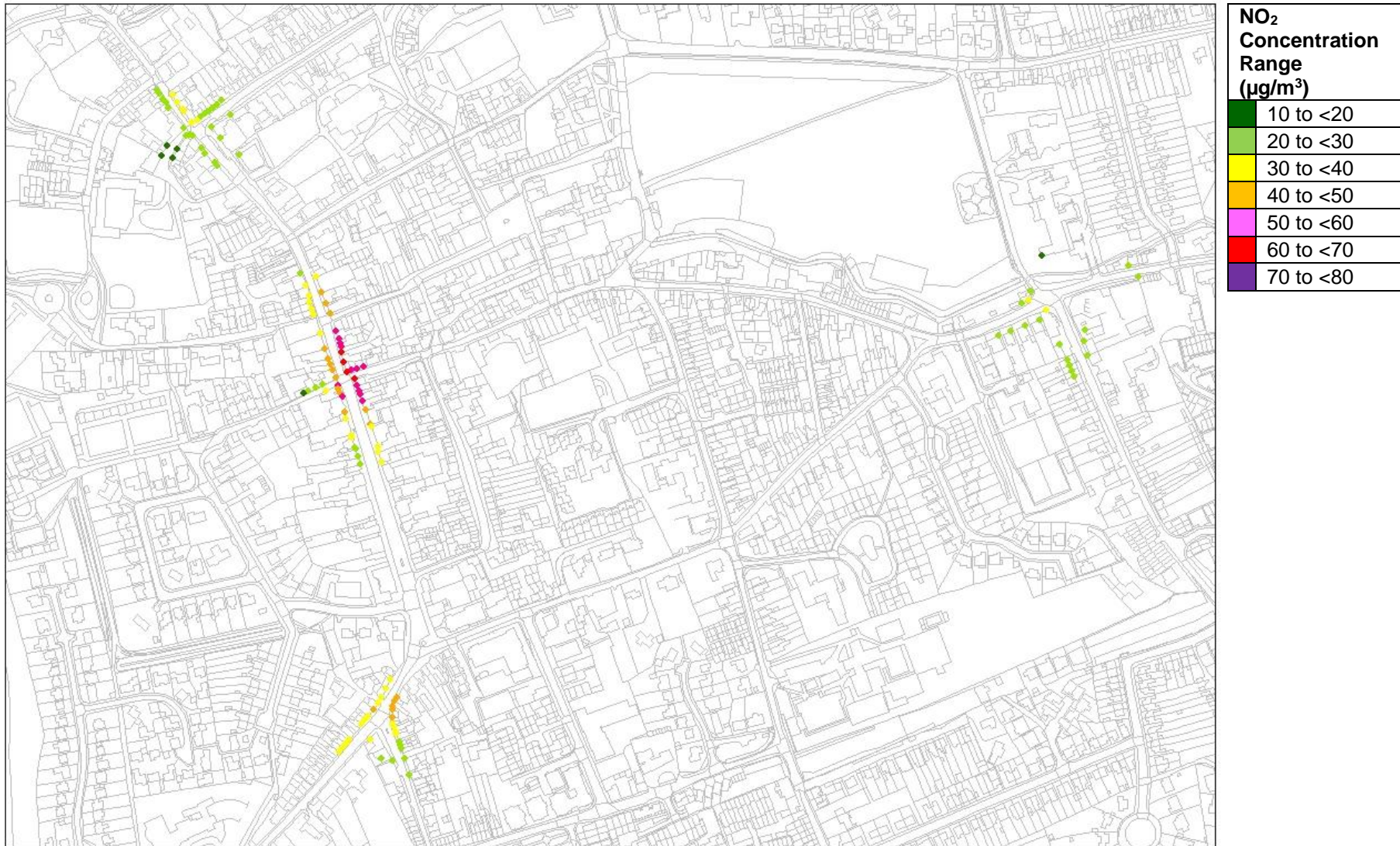
Figure 6-N: 2026 Full Scheme Scenario – Modelled Annual Mean NO 2 Concentrations (based on the LTT Methodology)
