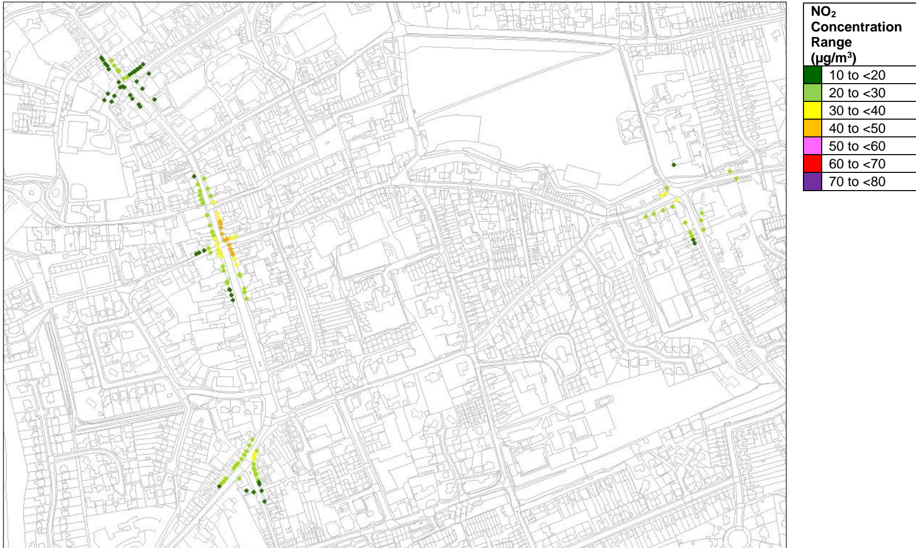
Figure 6-G: 2018 Full Scheme Scenario – Modelled Annual Mean NO 2 Concentrations (based on the LAQM TG09 Methodology)
